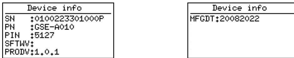
This page shows product information which is identical to the information on the product label. Also current software version is visible in this menu. Also the minimum and maximum internal measured temperatures (during lifetime) are shown here.
