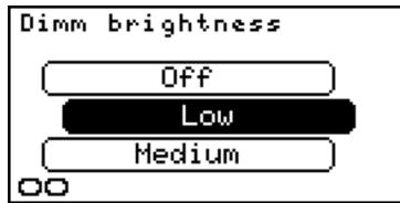
Select the low level of the backlight intensity. The Embion EMS Controller will reduce the backlight to the configured intensity when the buttons are not pressed for a while.
