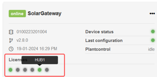
Figure 38: Licenses LED's in device status
